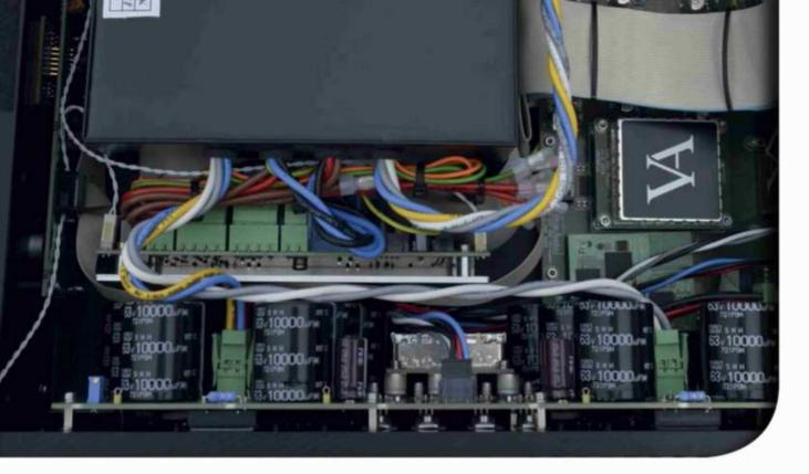
A POWER SUPPLY STORAGE/ SMOOTHING CAPACITANCE IS 216,000μF PER CHANNEL, UP FROM THE 120,000μF PER CHANNEL IN THE OLD RI-100. Volume level can be manually adjusted by using the 'Volume Up' button (the topmost of the three buttons to the right of the front panel display), or the 'Volume Down' button (the bottom-most of the three buttons). The button in the middle is 'Mute'.
